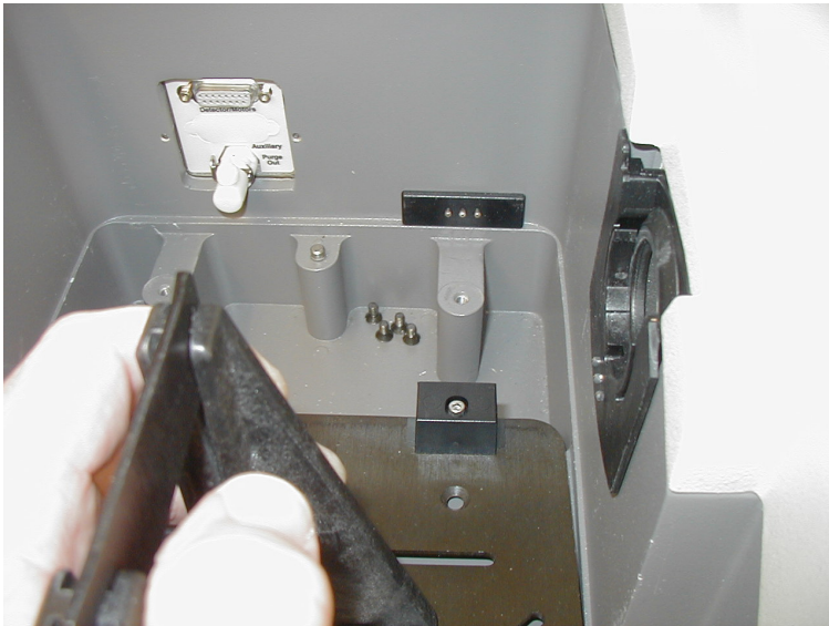
Bottom picture-removing Transmission sample accessory. To remove, pull up to clear pins. Two magnets hold the plate so that screws are not needed. Carefully pull back to remove.
